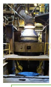
The primary smelting furnace within the pyrometallurgical facilities, the HENRI represents the centrepiece of the UrbanGold Flex recycling technology. The pyrometallurgical treatment carried out in this unit ensures an enrichment of valuable metals in a metallic phase and a separation of organic compounds and metallic impurities. The HENRI is designed to process up to 100% of e-waste fractions and therefore must meet the following requirements:
